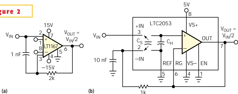
Practical implementations of the circuit in Figure 1 use the LT1167 (a) and the LTC2053 (b).
